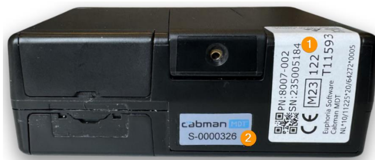
Figure 2-1: Seals that should be present on the Cabman MDT Box
