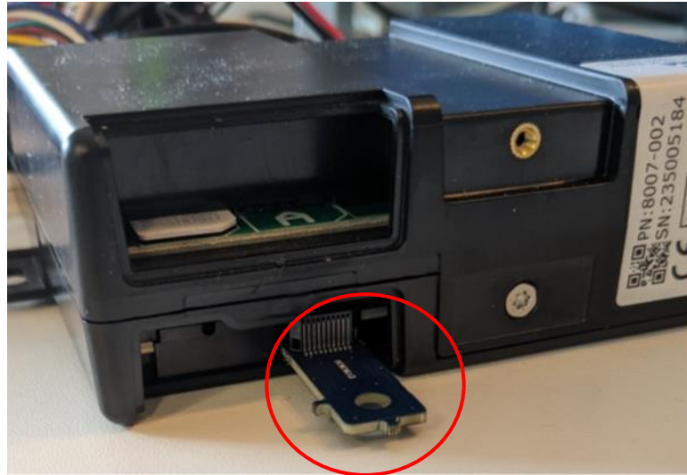
Figure 4-1: Inserting the COM3 dongle
