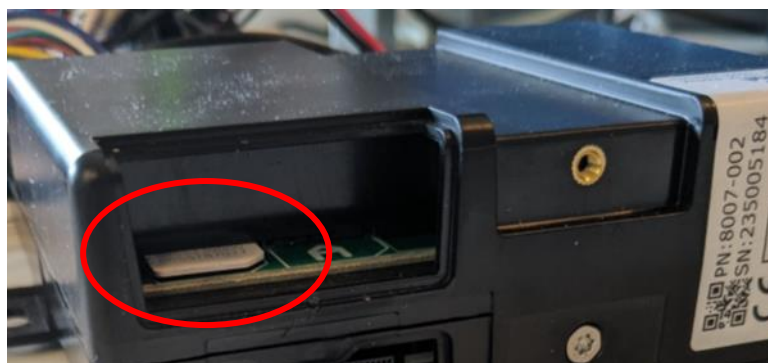
Figure 3-1: SIM-card location in the Cabman MDT Box
